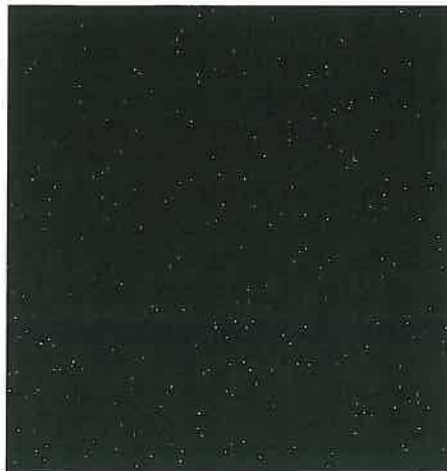
Figure 3: Damage tracks on film
