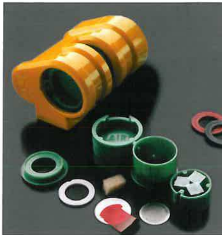
Figure 1: PAD body (yellow) and dosimeter head (green)
