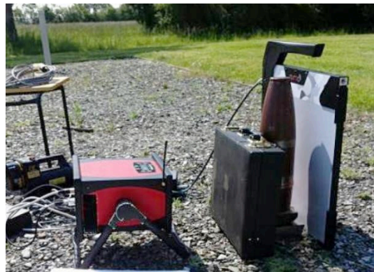
Figure 3. Inspection of IED (Improvised Explosive Device) by X-ray , by RadXman, CC BY-SA 3.0 , via Wikimedia Commons
