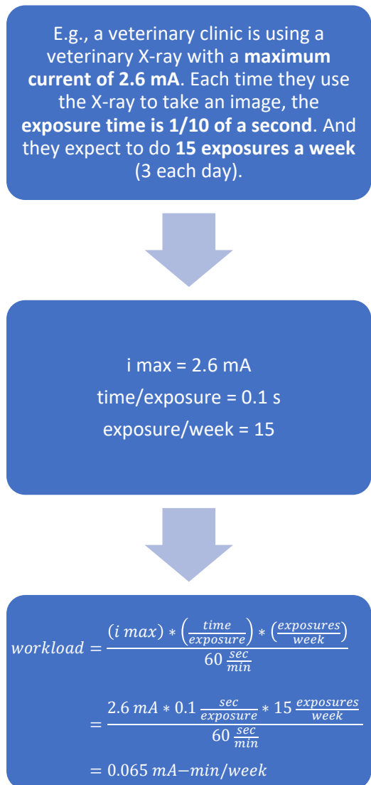
Figure 12. Sample Anticipated maximum workload calculation for a pulse-type X-ray source.
