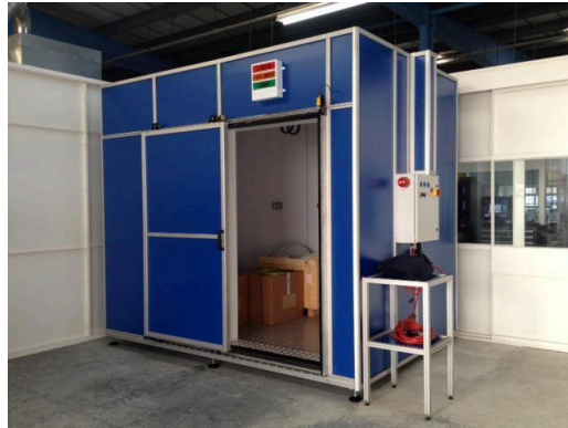
Figure 6. 200kV Large Walk-In X-ray Cabinet , images provided by kind permission of Euroteck Systems UK Limited, www.euroteck.co.uk
