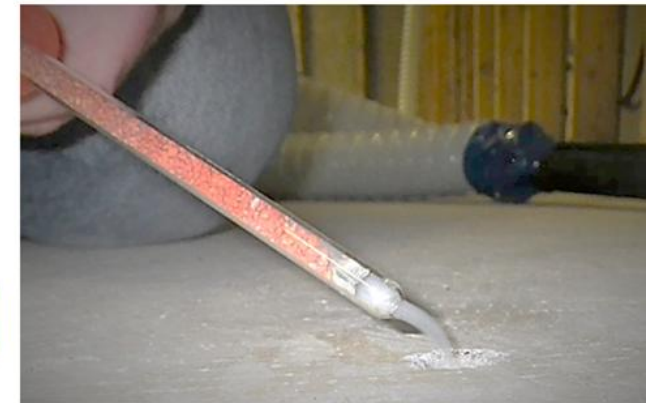
Negative pressure under the slab.
