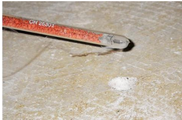
Positive pressure under the slab demonstrated with a smoke pencil
